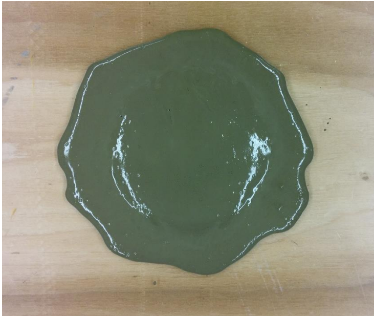
FIGURE 28 – SLUMP DIAMETER TEST P45-0-0
