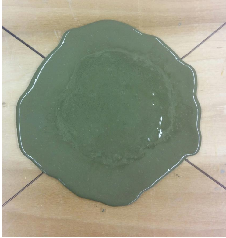
FIGURE 29 – SLUMP DIAMETER TEST P55-0-0
