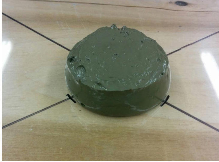
FIGURE 27 – SLUMP DIAMETER TEST P35-0-0
