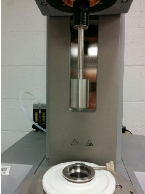
FIGURE 11 – BOB LOWERING INTO CO-CYLINDRICAL CUP
